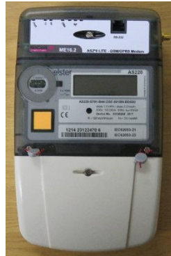
Single Phase Meters (Elster AS230/220) Future Use (L&G E460s)
