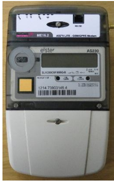
Single Phase Meters (Elster AS230/220) Future Use (L&G E460s)
